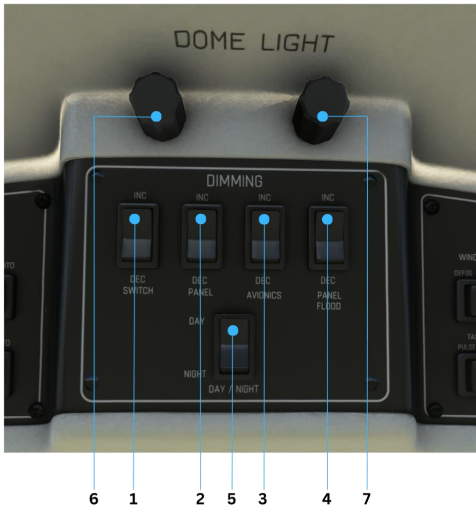
FIGURE 5-5: OVERHEAD DIMMING SWITCHES
