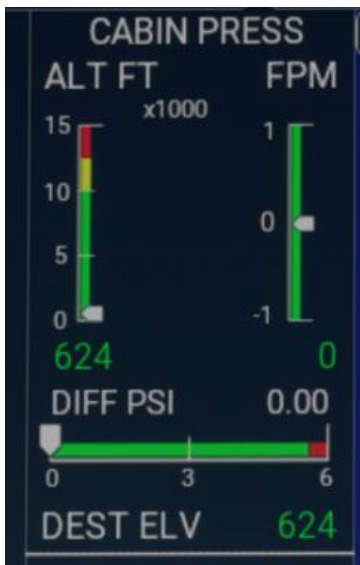
FIGURE 6-11: PRESSURISATION SYSTEM INSTRUMENTS
